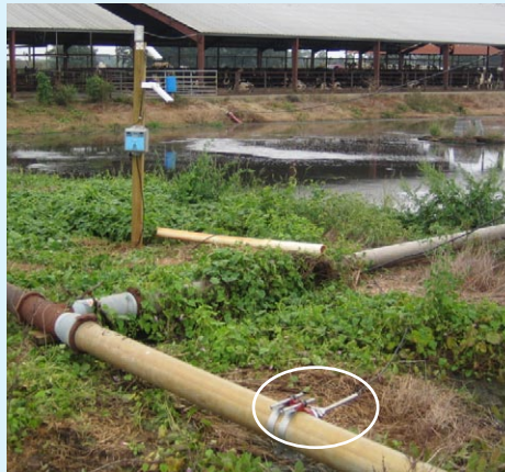
Figure 2: Typical dairy farm in southern Georgia, USA. Note the 2" insertion sensor in the foreground
