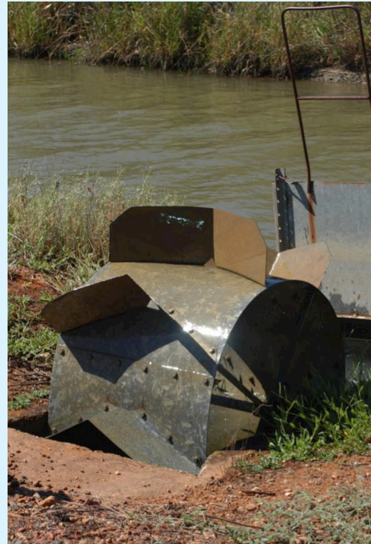
Figure 1: Dethridge wheel, note the large sharp vanes
