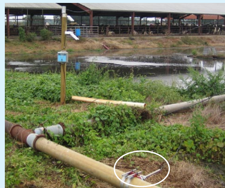
Figure 2: Typical dairy farm in southern Georgia, USA. Note the 2" insertion sensor in the foreground
