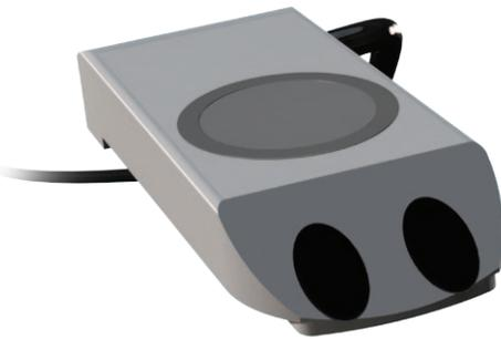
This sensor is used in open channels or pipes that run partially full. This sensor is used to measure depth (using a capacitive pressure diaphragm) and velocity. Access to the monitoring point is required for installation and maintenance.
