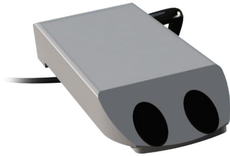
This sensor is used to measure velocity only in full pipes when access to the pipe is available and the pipe can be emptied when installation or maintenance is required. It can also be used in partially full pipes or open channels in situations where the user is measuring depth by a third party or ultrasonic depth sensor.
