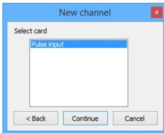
3. Select "**Pulse input**" and click "**Continue**". to complete the new channel. The "**Configure channels**" dialogue box will re-appear with the new channel listed.
