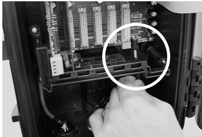
6. Once all the cables are connected the system should be fully tested. Assuming everything is connected and fully functional, in order to prevent insects and/or moisture damaging the system, the conduit entry point should be sealed with an appropriate product. Suitable sealants include:
