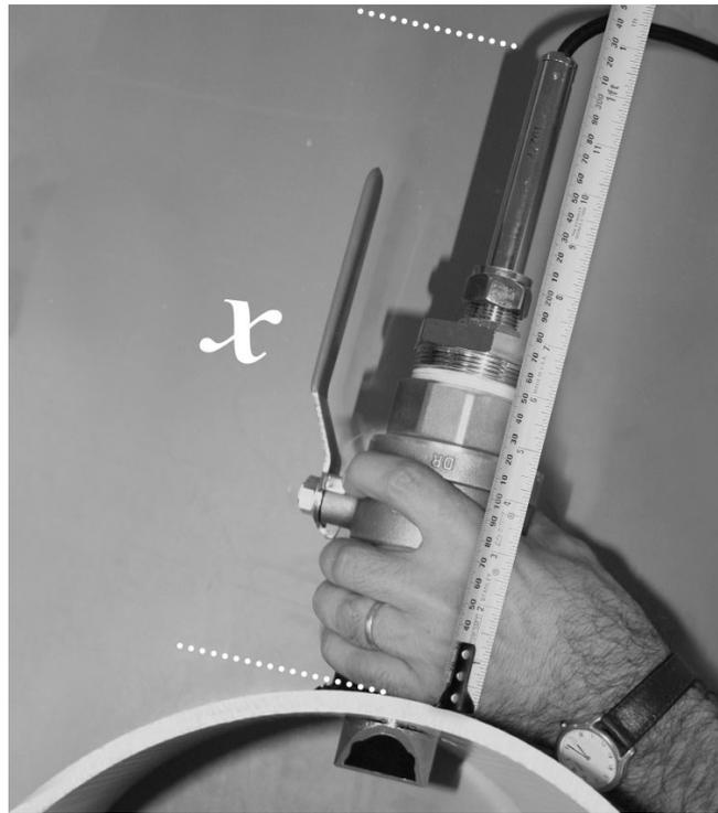
10. Now that the insertion depth is correct, rotate the sensor so that the grub screw at the top of the sensor shaft is roughly pointing in the direction of the longest straight section of pipe. Locate the plastic direction indicator tool that was supplied with the sensor. Clip the tool onto the stem of the insert sensor so that it is located in the two "blind holes" at the top of the stem with the grub screw facing the direction of the arrow.
