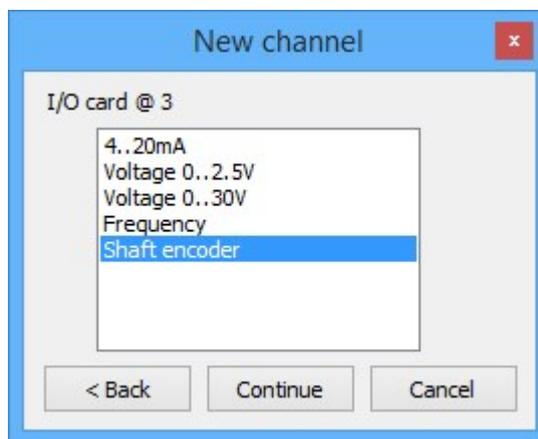
3. Select the "**Shaft encoder**" input type from the "**I/O Card @ Slot #**" list. Click "**Continue**" and then select "**Digital input #1**".
