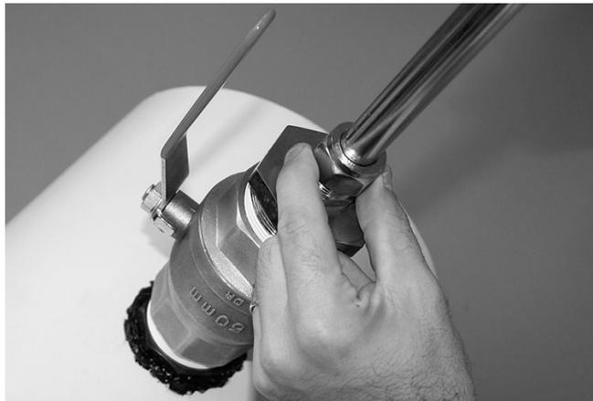
9. Open the valve fully and push the sensor head into the flow so it fully enters the stream without exposing any shaft. To get the sensor in exactly the right position you need to make the distance between the top of the sensor shaft to the top of the pipe wall the same as *value x*.
