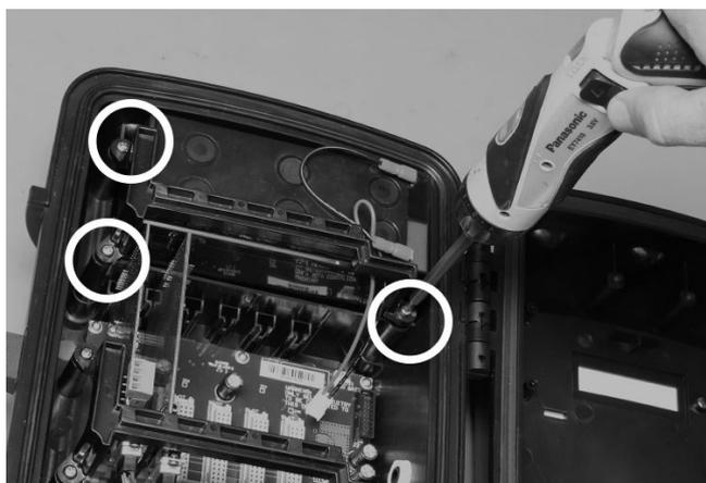
3. Carefully remove the battery from the main enclosure.
