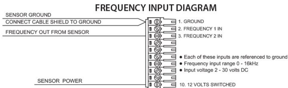
After completing the wiring, configure the sensor using FloCom+ (see [Add a new "Frequency" input type](#))
