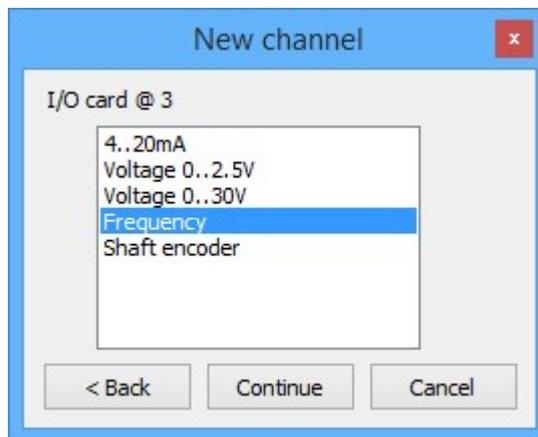
3. Select the "**Frequency**" input type from the "**I/O Card @ Slot #**" list. Click "**Continue**" and then select the appropriate *physically wired input* from which the named channel will receive its value.
