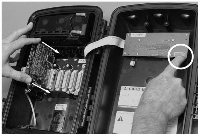
6. Replace the PCB clamping bracket ensuring that the slots in the underside of the bracket are aligned with the tops of all the cards. Fix the bracket into place with the three screws.
