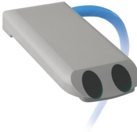
This type of configuration is used in full pipes when access to the pipe is available and the pipe can be emptied when installation or maintenance is required. Alternatively this sensor can be used in partially full pipes or open channels in conjunction with a MACE EchoFlo ultrasonic depth sensor.
