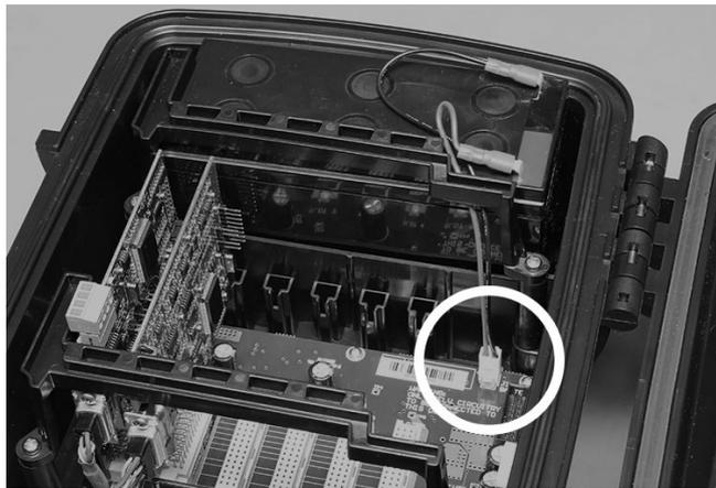
3. Unscrew the bracket that holds the cards in, using a Phillips #2 screwdriver.
