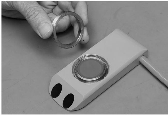
4. Remove the damaged ceramic depth sensor.
