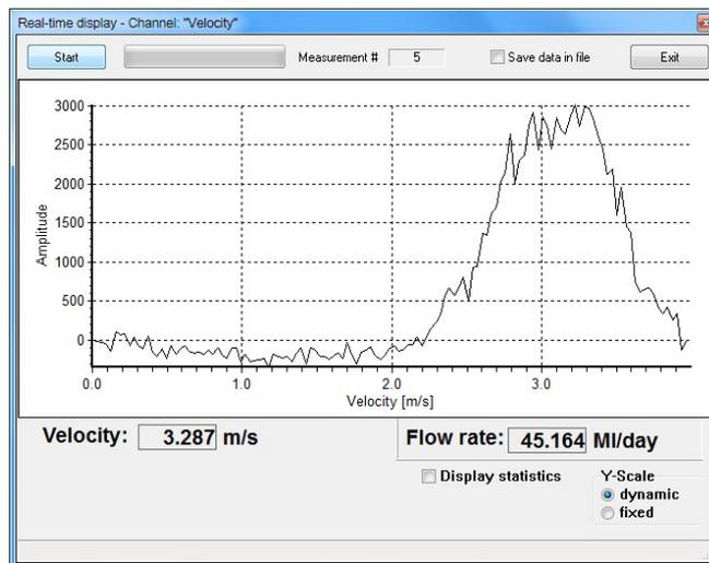
*This real-time graph displays a situation where the velocity range has not been set correctly for the site conditions. Velocities exceeding the set range are not being captured. Furthermore, the velocity readings that are missed WILL cause the processing electronics to alias and the overall average velocity calculated will be unreliable. The range MUST be set to at least double the average velocity. This enables all velocities across the range to be captured.*
