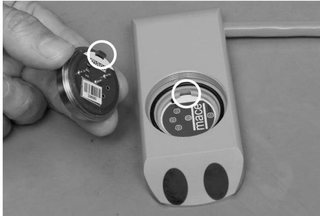
4. Place the ceramic module so that it sits flush with the o-ring.
