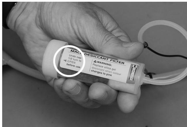
2. Unscrew the cap half a turn, until the mark on the cap is in line with the arrow on the label.
