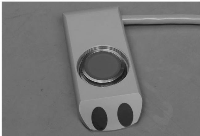
5. Gently start to screw the "locking ring" in by hand. Only turn it one or two turns, just enough to get the thread 'started'.
