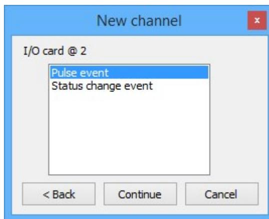
3. Select either the "**Pulse event**" or "**Status change event**" input type from the "**I/O Card @ Slot #**" list. Click "**Continue**" and then select "**Digital input #3**" from which the named channel will receive its value.
