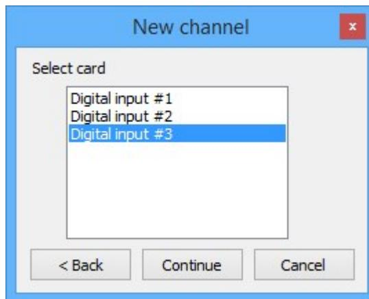
3. Select the appropriate *physically wired input* from which the named channel will receive its value.
