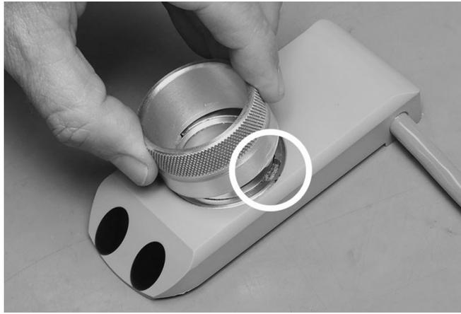
3. Unscrew the locking ring using the tool, and remove completely.
