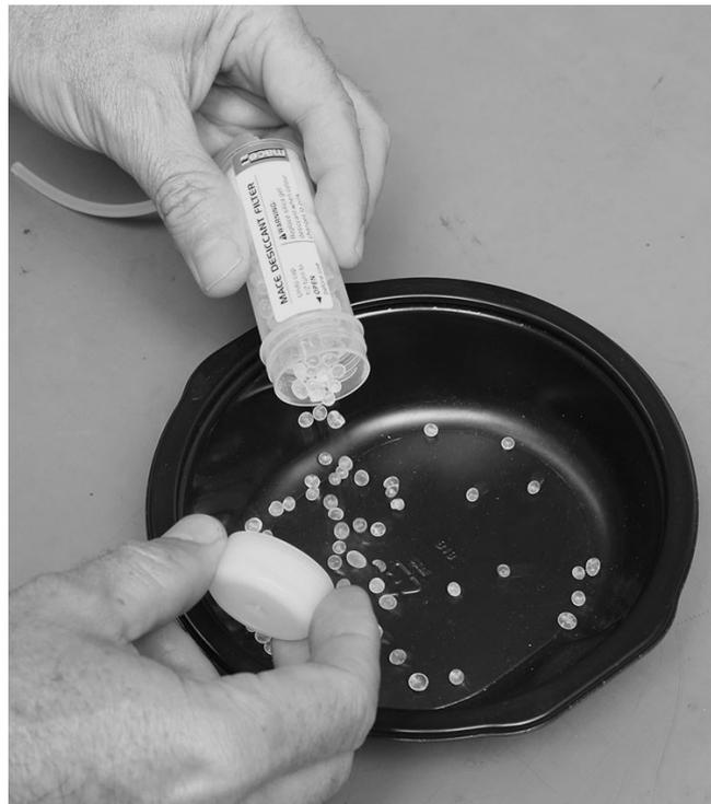
3. Add new crystals (MACE Part No. 590-009) to the filter chamber to the top of the tube level.
