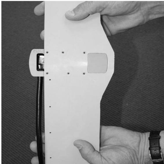
3. You should see six countersunk holes in the strap. Fit the six screws supplied (M3 x 8 mm Phillips head countersunk 304 s/s).
