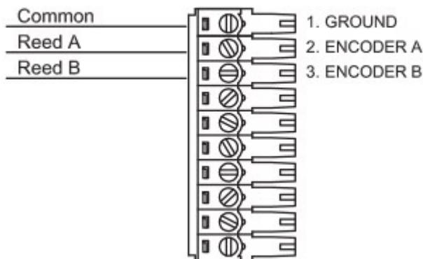
After completing the wiring, configure the sensor using FloCom+ (see [Add a new "Shaft encoder input" input type](#))
