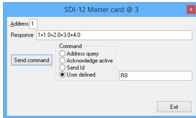
In the 2nd example, the sensor on Address "1" of the SDI-12 bus has responded to a "R0" command with the Response "1+1.0+2.0+3.0+4.0".
