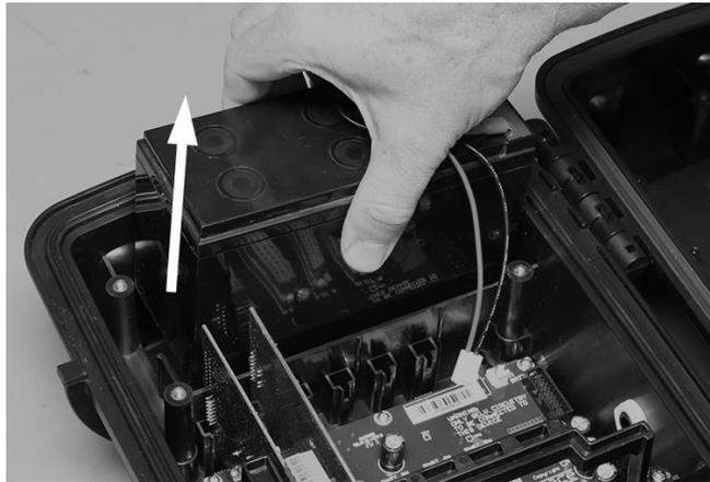
4. Disconnect the battery cable from the battery terminals.
