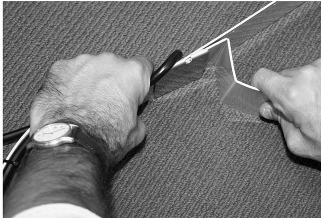
11. Hold the 'Z' with one hand, the sensor with the other and place the assembly into the pipe reaching as far as is comfortable. Ensure that the sensor is parallel to the flow and in the bottom part of the pipe, off set to either side (if there is a build up of debris the sensor will not get covered)
