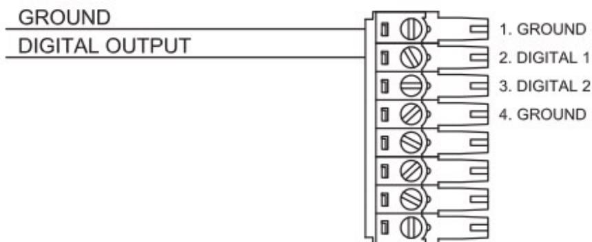
After completing the wiring, configure the output using FloCom+ (see ["Pulse" - output type](#))
