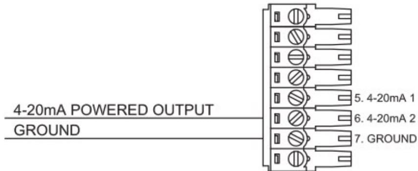
After completing the wiring, configure the output using FloCom+ (see "4-20mA" - output type)
