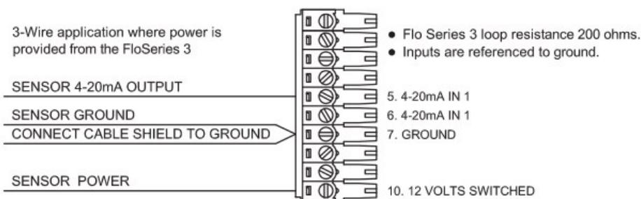
After completing the wiring, configure the sensor using FloCom+ (see [Add a new "4-20mA" input type](#))
