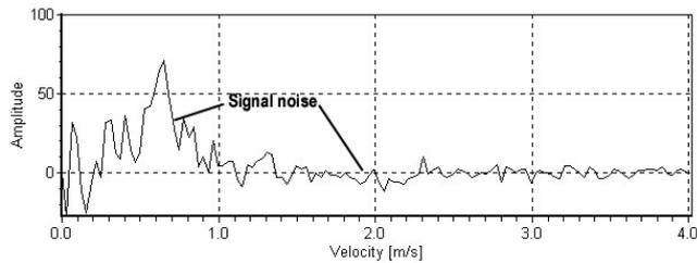
*In the figure above signal noise can be seen on the velocity spectrum graph as low signal strength echoes. In the graph above you can see that the signal noise has an approximate amplitude value of 75. Therefore, by setting a threshold of say 100, this noise will be ignored in the computation of average velocity. The user should be careful however, at sites where signal strength is inherently lower, a peak threshold that is set too high could mean that true velocity readings are discarded.*
