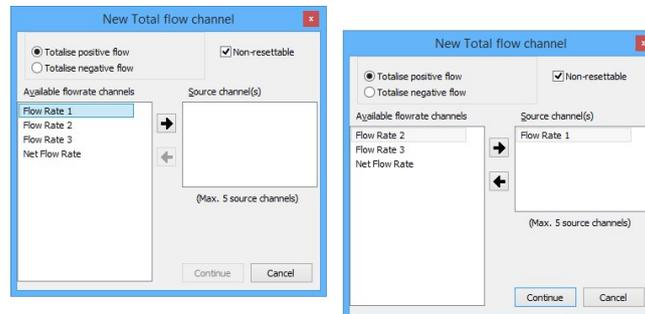
1. From the "**Available flowrate channels**" list, highlight the "**Flowrate**" channel from which the "**Total flow**" channel will receive its value. Click the "**Right arrow**" and the channel will appear in the "**Source channel(s)**" list. A maximum of five flowrate channels can be totalised together.
