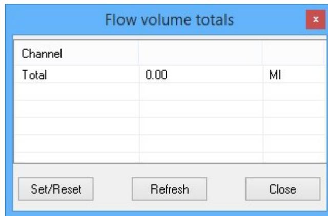
If the AgriFlo XCi device has not been started, the “**Set/Reset**” button will be active and the totalised reading can be changed.
