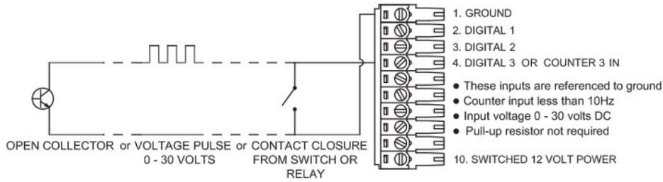
After completing the wiring, configure the sensor using FloCom+ (see [Add a new "Binary" channel type](#) or [Add a new "Input pulse total" channel type](#))
