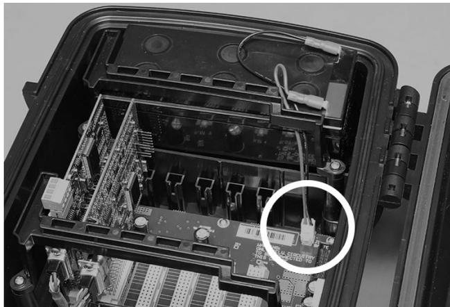
2. Use a #2 Phillips head screwdriver to remove the three screws which fasten the battery bracket to the main enclosure.
