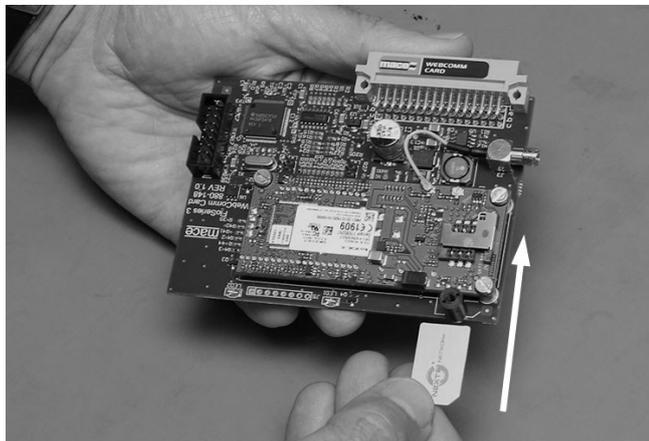
3. Slide the SIM card into the slot until it is fully seated and behind the small black "**holding pin**".
