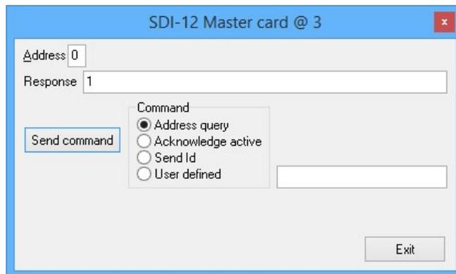
*In the example, the sensor has responded to an "Address query" with Address "1".*
