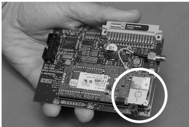
4. Screw the supplied antenna onto the SMA antenna connector.
