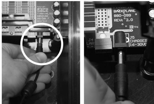
2. Alternatively, if a DC source other than a MACE charger is used, this is terminated using the same three-pin connector as for the [solar panel](#).
