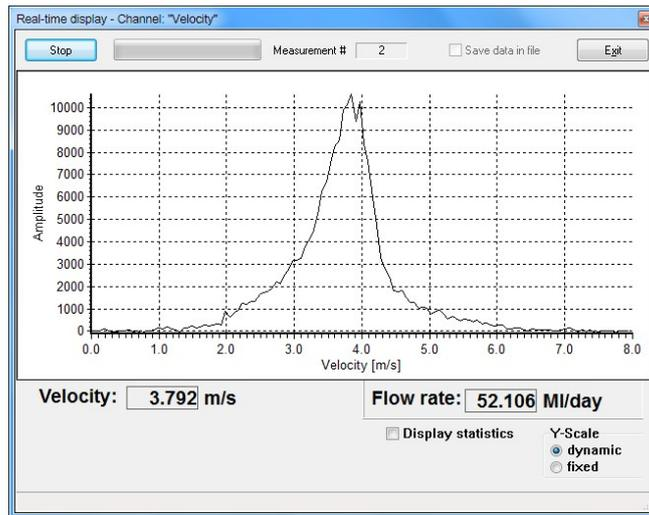
*This real-time graph displays an ideal "bell shape" centred across the velocity range. The range has been set to double the average velocity. This enables all velocities across the range to be captured.*
