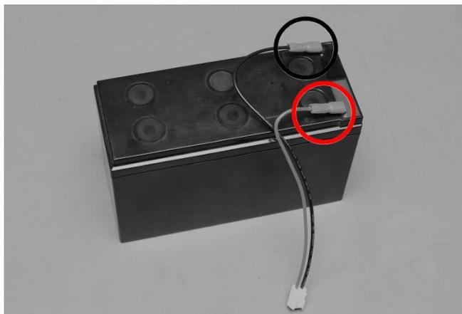
2. Place the battery in the main enclosure and hold it in place.
