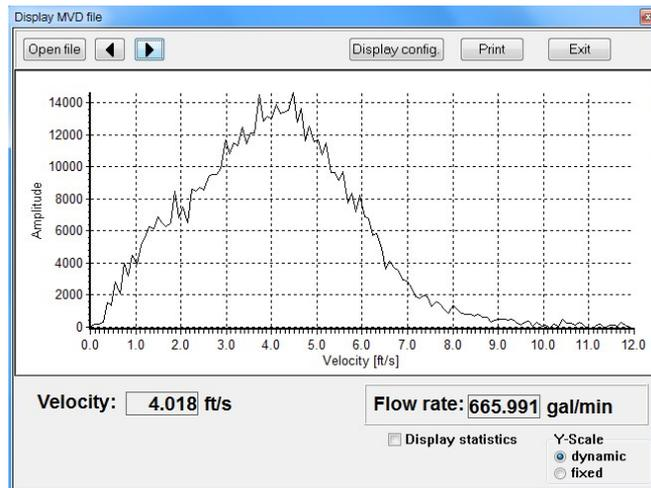
*This real-time graph displays velocities captured by a sensor at a wastewater pump site. Pumped flows typically exhibit graphs with a broader base than gravity flows.*
