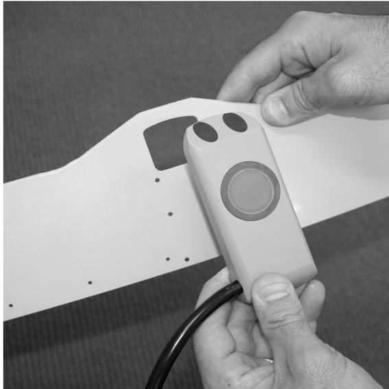
2. Turn the whole assembly over. Make sure the cut out in the strap sits down around the 'foot' on the sensor.
