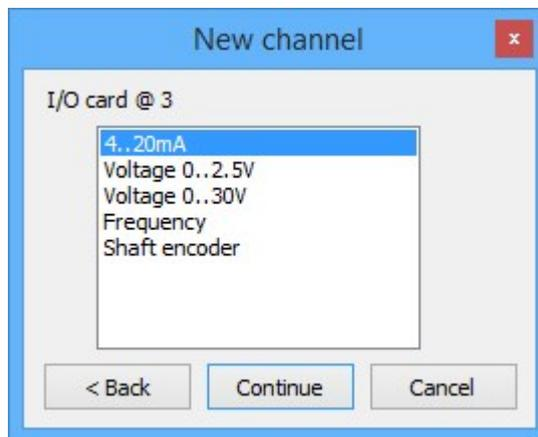
3. Select the "**4..20mA**" input type from the "**I/O Card @ Slot #**" list. Click "**Continue**" and then select the appropriate *physically wired input* from which the named channel will receive its value.
