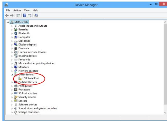
5. Double-click on the "**USB Serial port**" icon and open its "**Properties**" dialogue box. The device status box confirms there are no installed drivers
