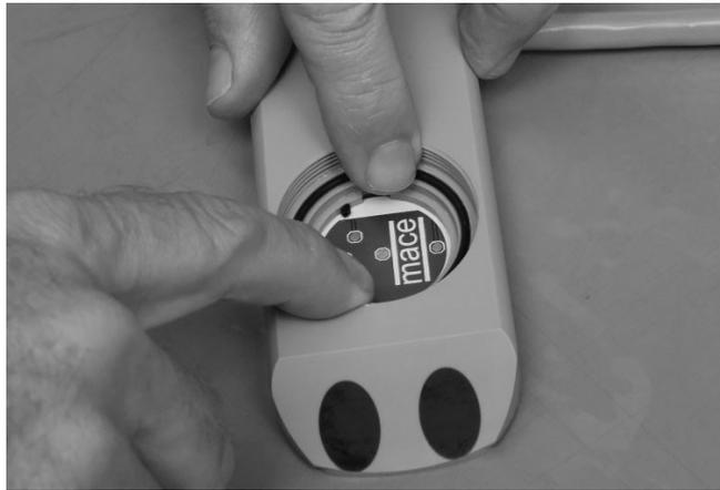
3. Find the "**locating pin**" on the base of the ceramic module and the matching "**aperture**" within the area/velocity sensor.
