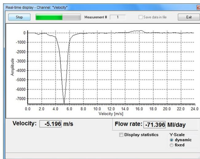
*This real-time graph displays velocities captured by a sensor facing downstream. Although the amplitude of the graph is negative the calculated average velocity is positive because the "Sensor orientation" has been set to "Downstream" in the Doppler module configuration.*
