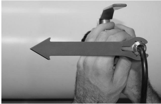
12. Tighten the 3/4" gland nut to lock the sensor in place. **Do not use thread sealant on the 3/4" gland nut.**
