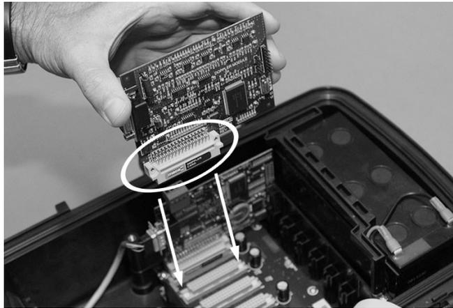
5. **Ground yourself again.** Your finger must remain grounded on the screw whilst carefully inserting the card into any spare slot. Take care to align the pins of the two connectors together. There is a slot at the top of the card area that helps the alignment process. Ensure that the card is contained within this slot and press down firmly to ensure that it is fully seated.
