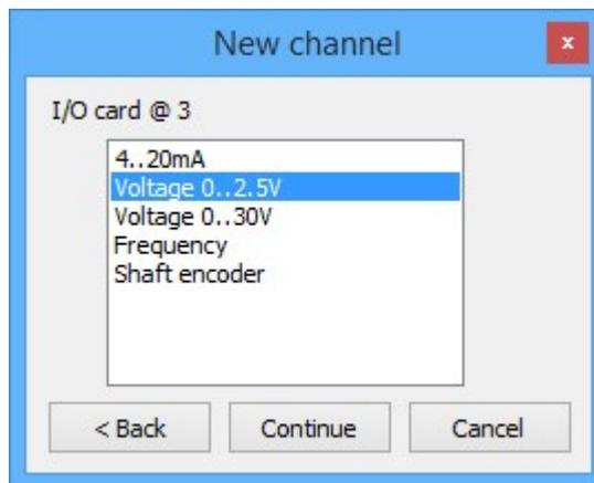
3. Select the "**Voltage**" input (range) required from the "**I/O Card @ Slot #**" list. Click "**Continue**" and then select the appropriate *physically wired input* from which the named channel will receive its value.
